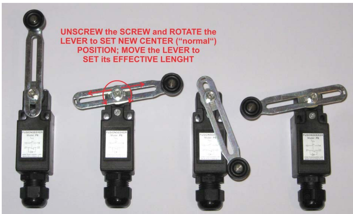
Figure 3: Fully adjustable lever of the Fusionseeker P6 limit switch
